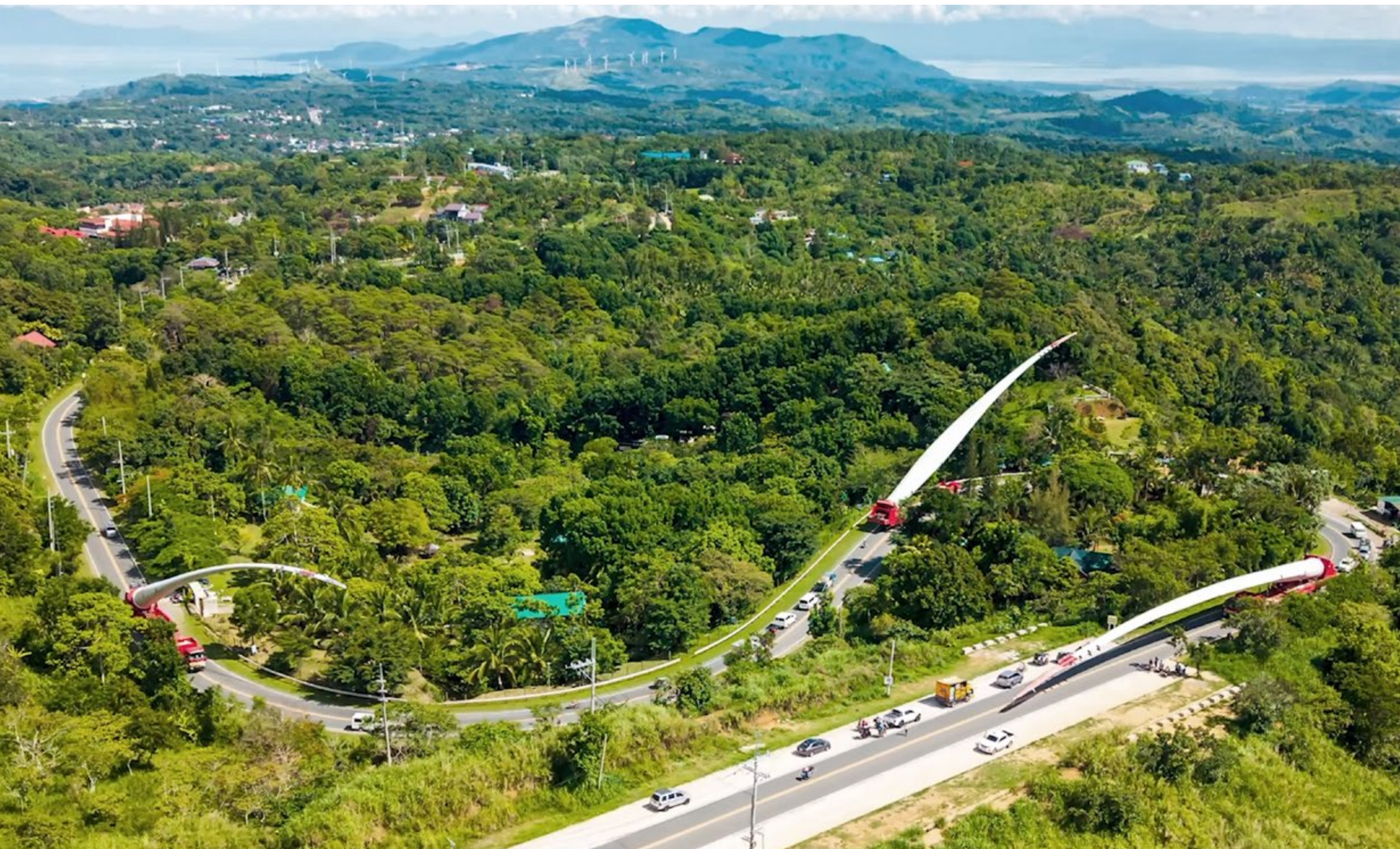
Transporting Tanay Wind Power Project's 90-meter wind turbine blades along Marilaque Highway
